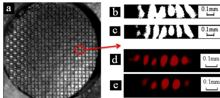
Figure 5. (a) Ni mesh and fringe patterns with different applied pressures: (b) 0 kPa (0 psi) (c) 131 kPa (19 psi) at RT, and (d) 34.47 kPa (5 psi) (e) 103.42 kPa (15 psi) at 800°C
