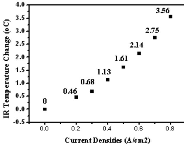
Figure 11. Steady-state surface temperature changes of button cell at different loading current densities with 100 sccm H<sub>2</sub>/3 vol.% H<sub>2</sub>O (Surface temperature T = 800.06 °C at i = 0 A/cm<sup>2</sup>)
