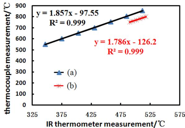
Figure 10. Steady-state IR temperatures calibration based on a thermocouple measurement under different environments: (a) air and (b) hydrogen.
