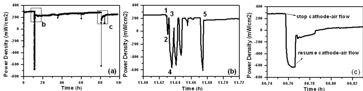
Figure 6 (a) Button cell power density plot during pressure changes (b) Effect of cathode side air pressure, (c) Effect of cathode side air flow rate
