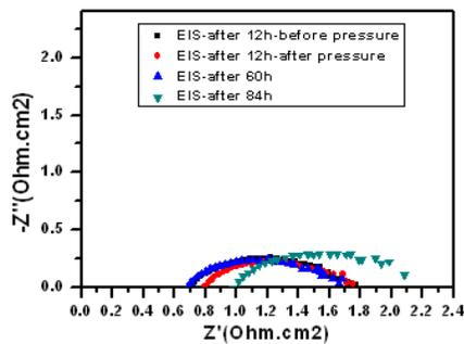
Figure 8. Impedance plots for SOFC operating at 800 °C, 0 V and 100 sccm H<sub>2</sub>/3vol.% H<sub>2</sub>O
