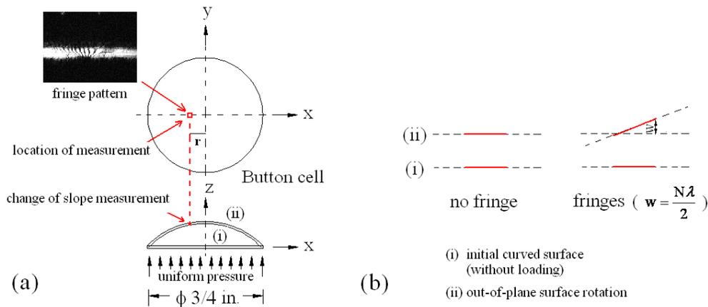
Figure 2. (a) Button cell under uniform pressure with corresponding fringe patterns on a spot location of the Ni wire mesh, (b) Button cell surface rotation before and after loading
