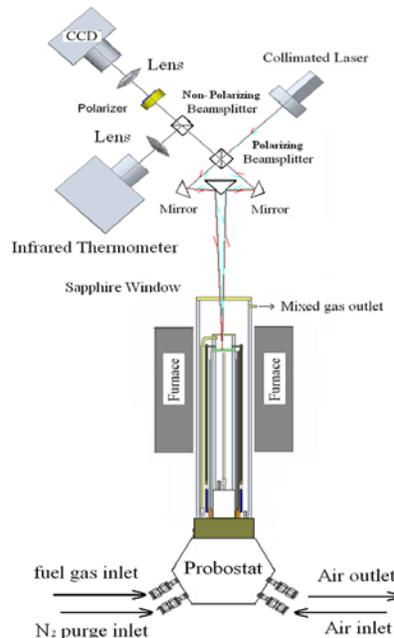
Figure 1. NexTech Probatat<sup>TM</sup> integrated with Sagnac interferometry and IR thermometer
