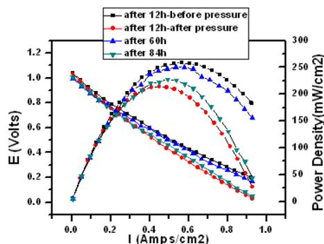
Figure 7. I-V curves of SOFC operating at 800 °C
