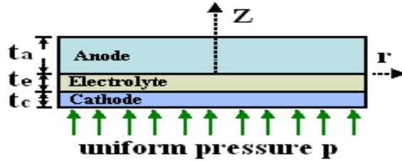
Figure 3. Button cell modeled as a three-layered thin membrane
