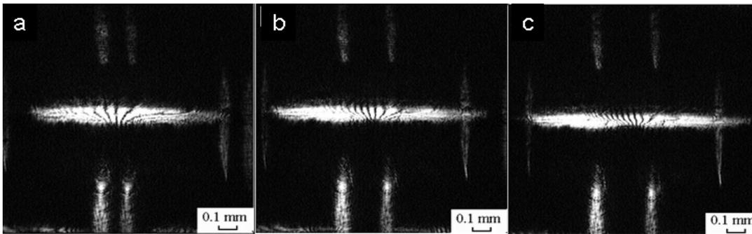
Figure 4. Fringe patterns on Ni mesh at RT with different applied pressures: (a) 0 kPa (0 psi), (b) 48.26 kPa (7 psi), and (c) 89.63 kPa (13 psi)
