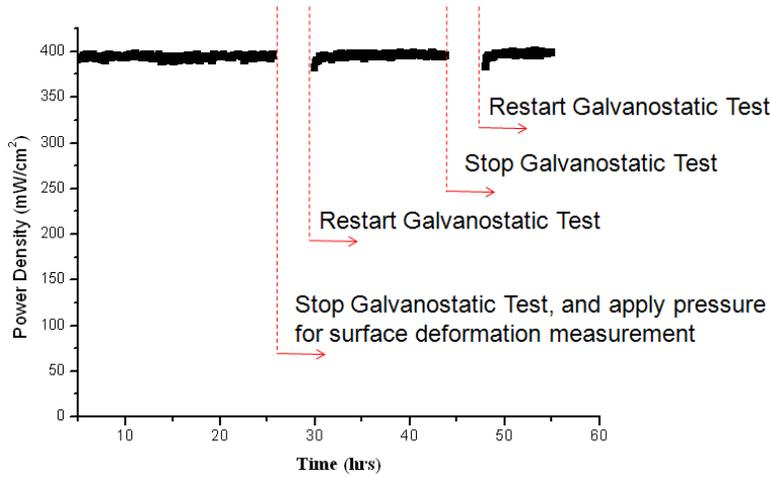
Figure 9.1 Remedy of cathode-air interruption on performance of SOFC with 100 sccm H<sub>2</sub>/3vol.% H<sub>2</sub>O at 800 °C (0.5 A/cm<sup>2</sup>)
